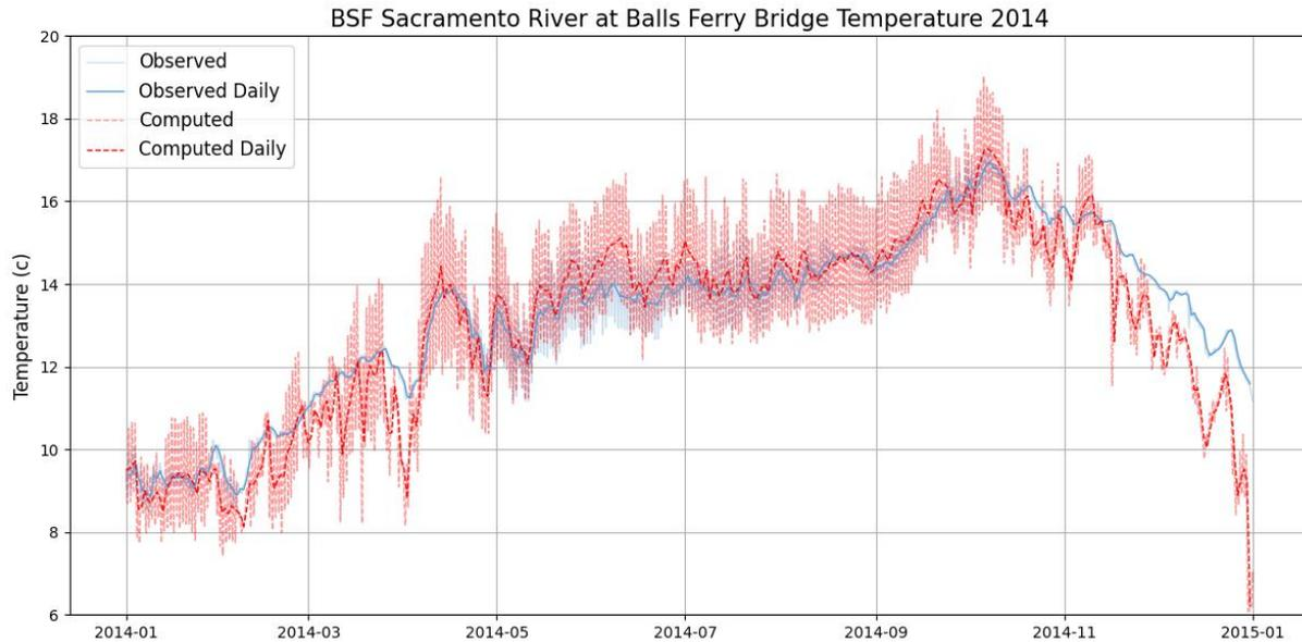
Figure 4-30. Simulated and observed temperatures at BSF: 2014.
