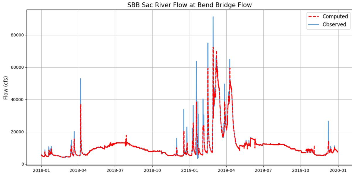
Figure 4-48. Simulated and observed hourly flows at Bend Bridge: 2018-2019.
