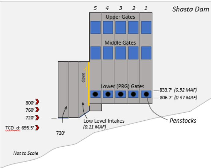
Figure 3-2. Shasta Dam TCD showing low-level intake structure (looking downstream) represented with three individual point sinks at 800 ft (243.8 m), 760 ft (231.7 m), and 720 ft (219.5 m) and the addition of the TCD\_d point sink at 695.5 ft (212.0 m).
