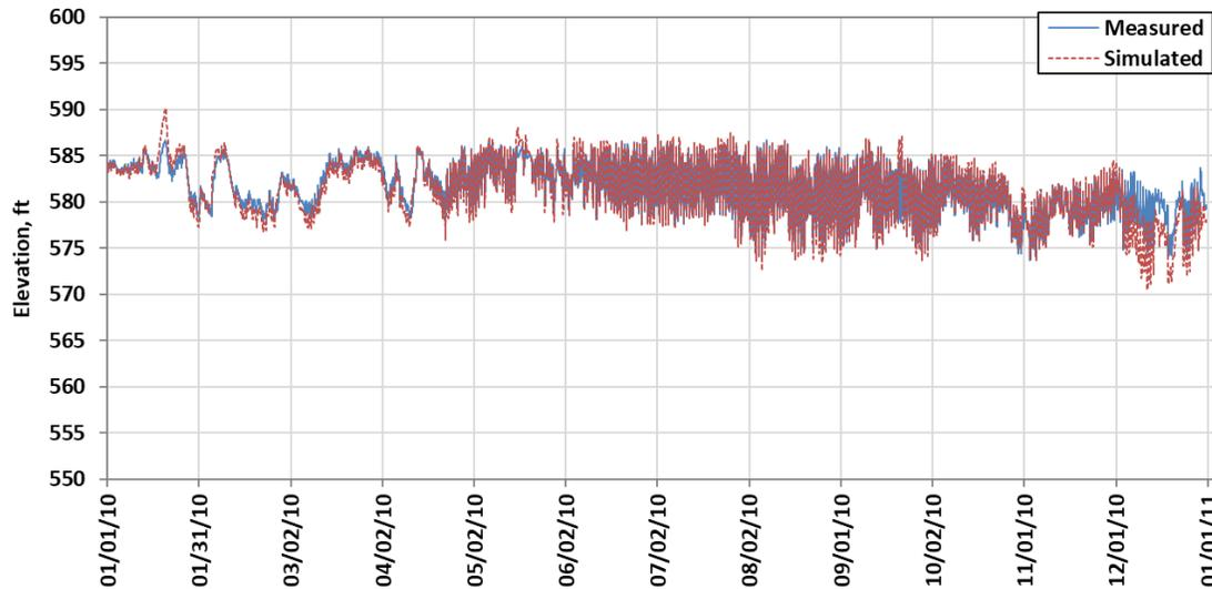
Figure 4-5. Simulated versus measured Keswick Reservoir stage (msl). Year 2010.
