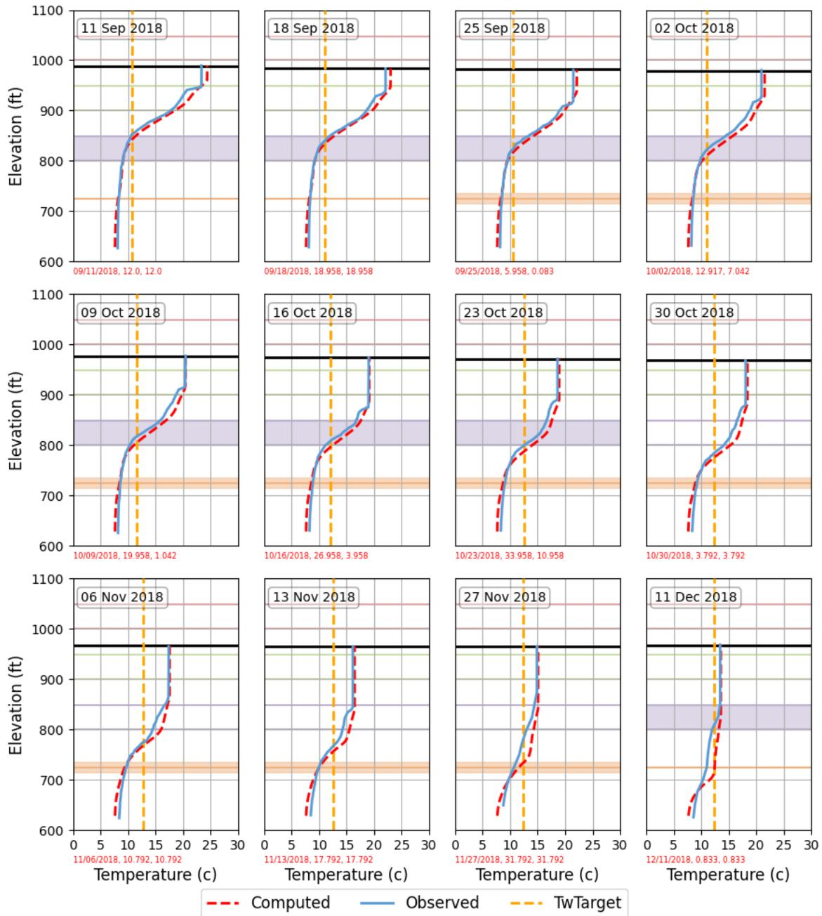
Figure 4-41. Simulated and observed temperature profiles and TCD gate positions during 2018 (3/3).
