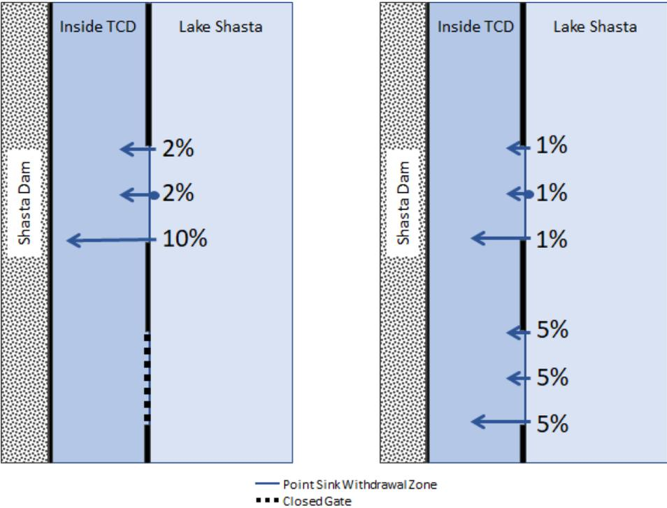
Figure 3-1. Minimum flow fractions (MFF) using upper and middle levels as an example for single active level (left), and two active levels (right).
