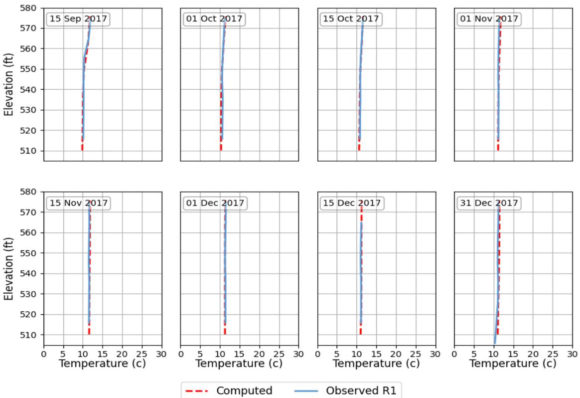
Figure 4-20. Keswick Reservoir simulated and observed temperature profile comparisons, 2017. Profiles data are collected approximately 0.1 miles upstream from dam.
