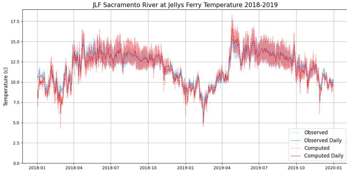
Figure 4-51. Simulated and observed temperatures at JLF: 2018-2019
