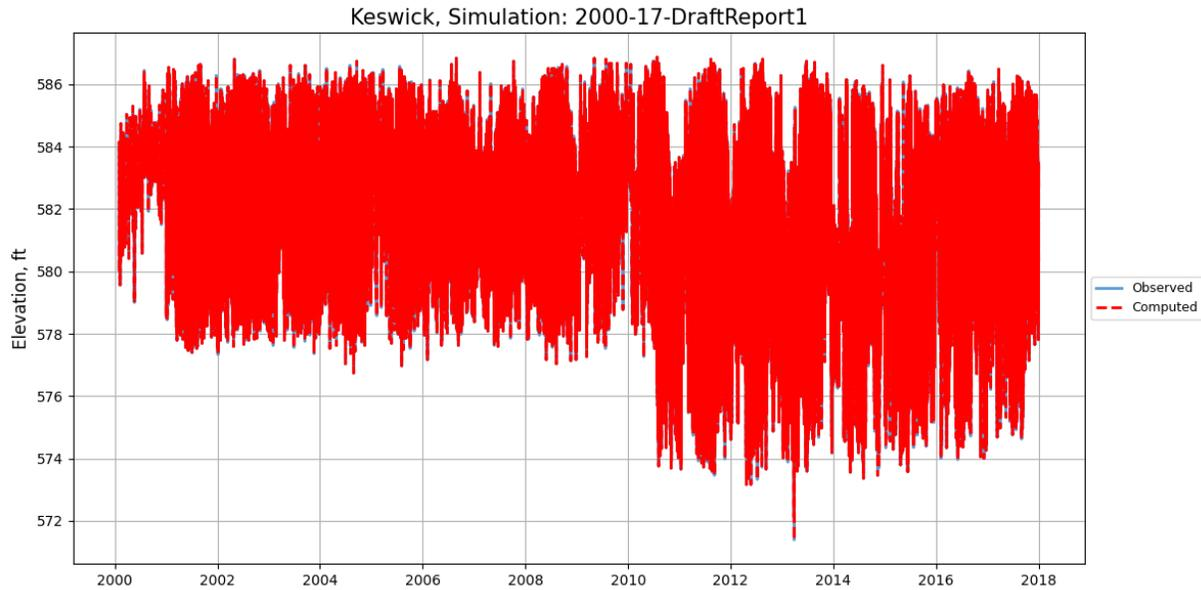
Figure 4-18. Keswick Reservoir simulated and observed water surface elevation, 2000-2017.
