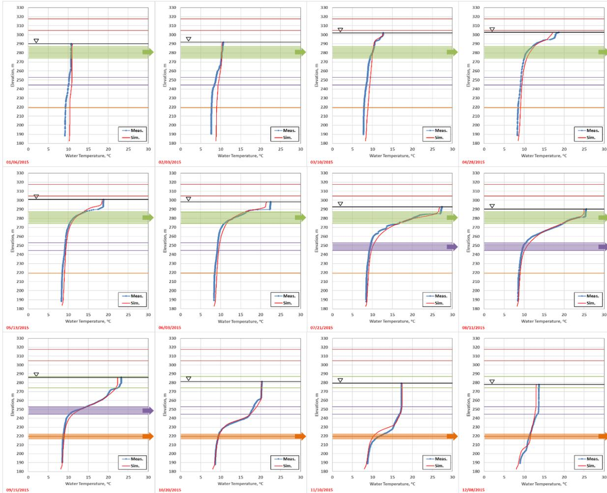
Figure 4-3. Simulated versus measured temperature profiles upstream of Shasta Dam: 2015.
