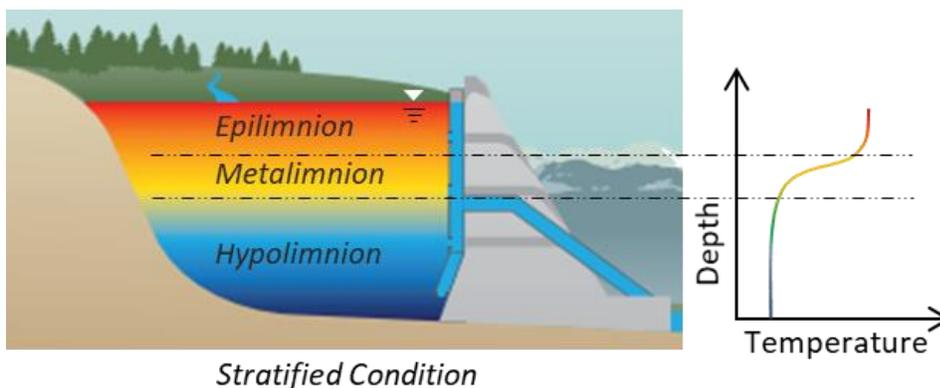
Figure 2-3. Representative seasonal stratification for a large reservoir, showing the epilimnion, metalimnion, and hypolimnion and associated thermal profile.
