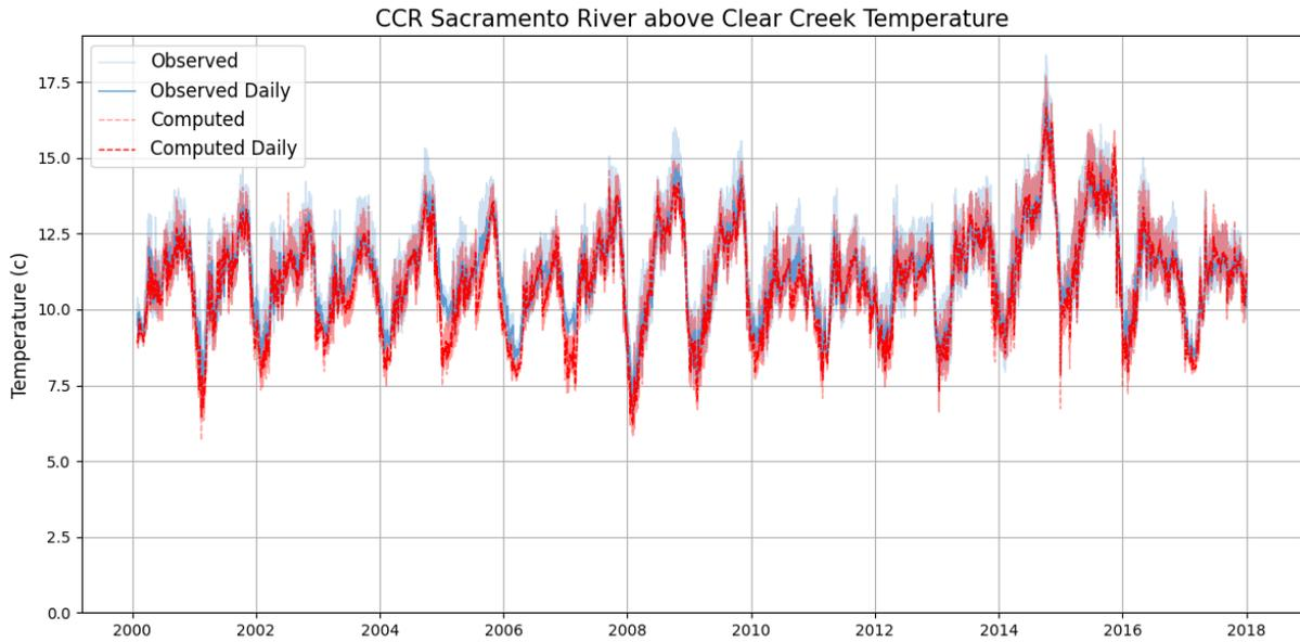
Figure 4-25. Simulated and observed temperatures at CCR: 2000-2017.
