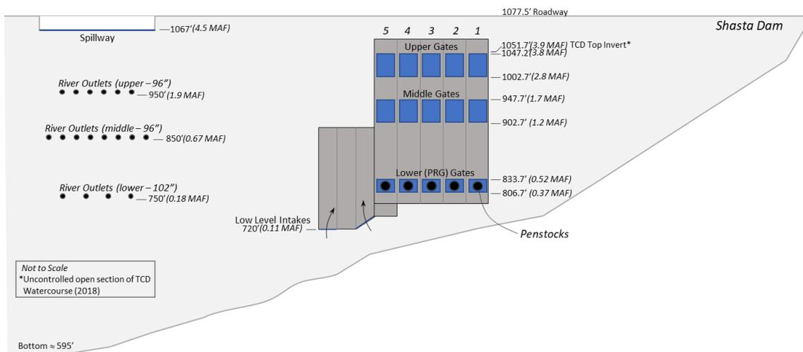
Figure 2-2. Shasta Dam outlet works (left) and Temperature Control Device (right) looking downstream. Powerhouse units 1 through 5 are shown for reference.
