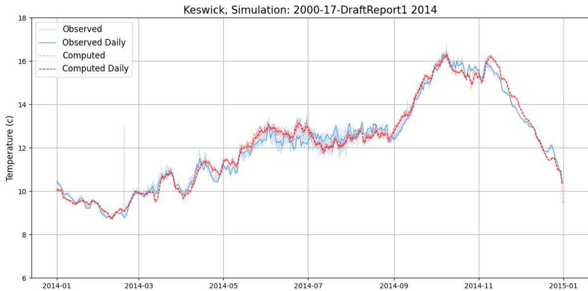
Figure 4-22. Simulated and observed outflow temperatures from Keswick Dam: 2014.
