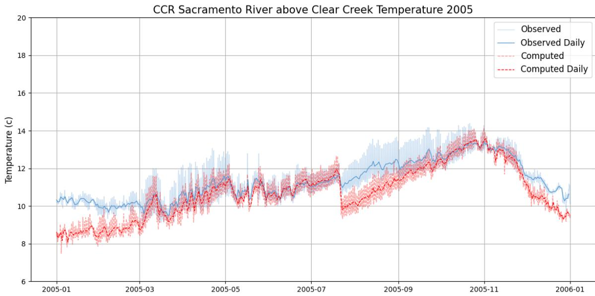
Figure 4-26. Simulated and observed temperatures at CCR: 2005.
