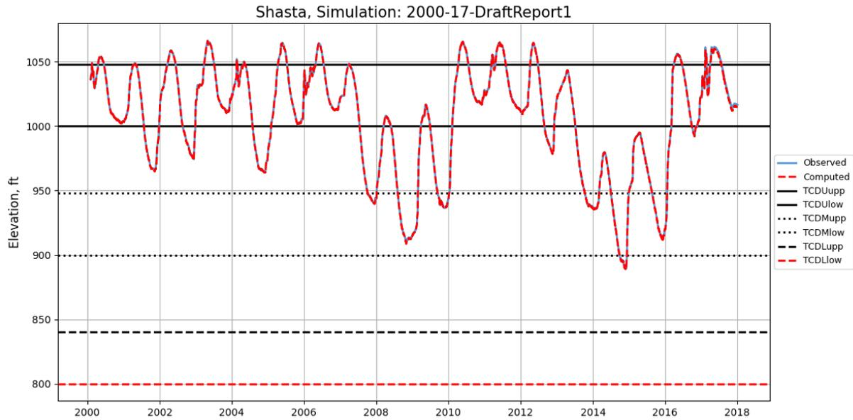
Figure 4-10. Shasta Lake simulated and observed water surface elevation, with TCD gate elevations, 2000-2017.
