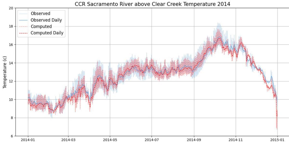
Figure 4-27. Simulated and observed temperatures at CCR: 2014.
