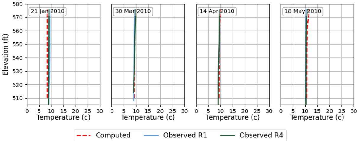
Figure 4-19. Keswick Reservoir simulated and observed temperature profile comparisons, 2010. Station R1 and R4 are 2.3 and 1.5 miles upstream from dam, respectively.
