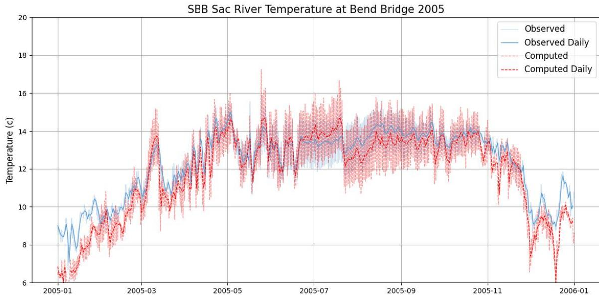
Figure 4-35. Simulated and observed temperatures at BND: 2005.
