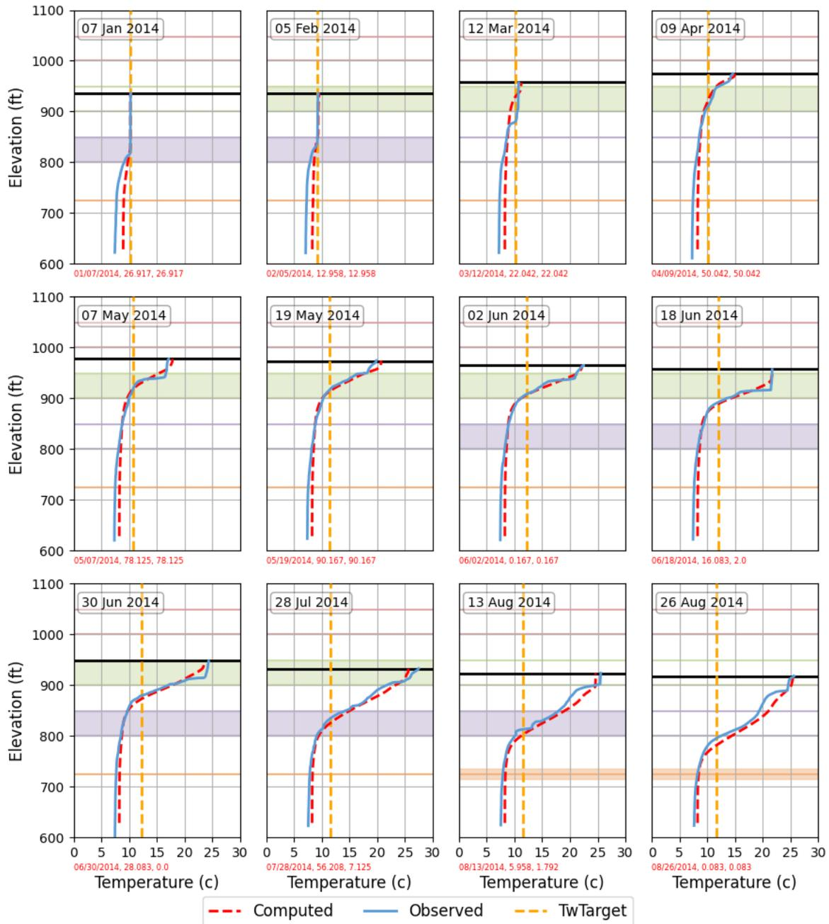
Figure 4-12. Simulated and observed temperature profiles and TCD gate positions during 2014 (1/2).
