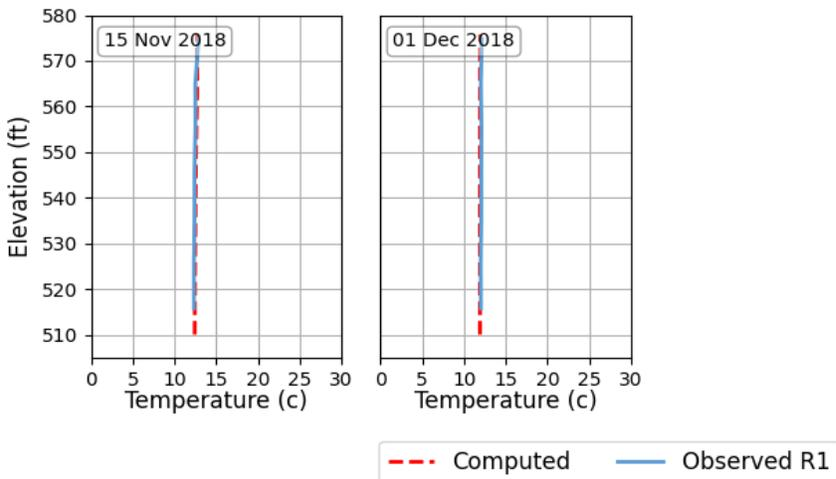
Figure 4-46. Keswick Reservoir simulated and observed temperature profile comparisons, 2018. Profiles data are collected approximately 0.1 miles upstream from dam (2/2).
