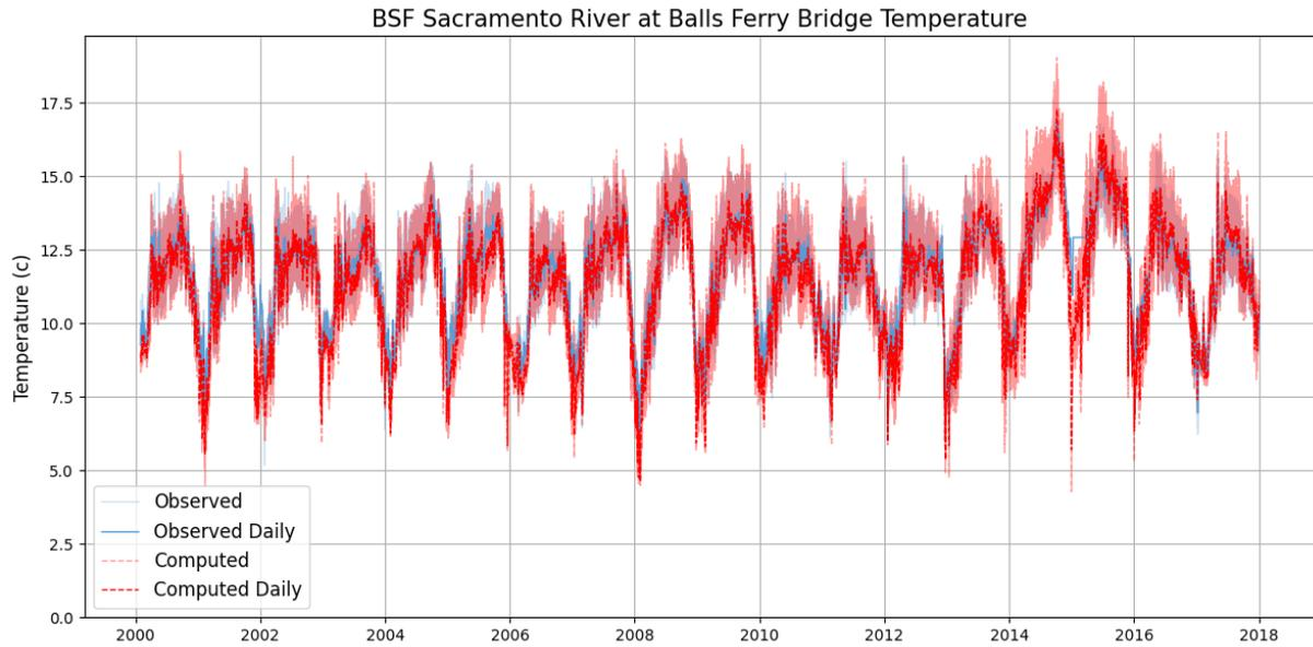
Figure 4-28. Simulated and observed temperatures at BSF: 2000-2017.
