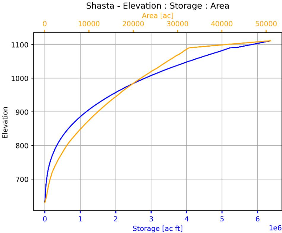
Figure 3-3. Shasta Lake Elevation-Storage and Elevation-Area Curves.
