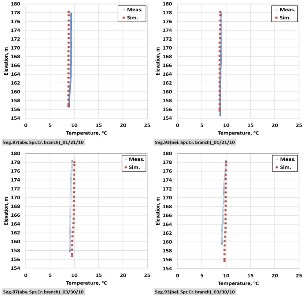
Figure 4-7. Simulated versus measured temperature profiles. 01/21 (top) and 03/30 (bottom), Year 2010.
