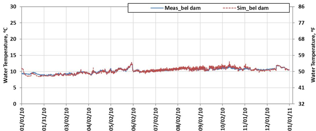
Figure 4-9. Simulated versus measured temperature below Keswick Dam. Year 2010.
