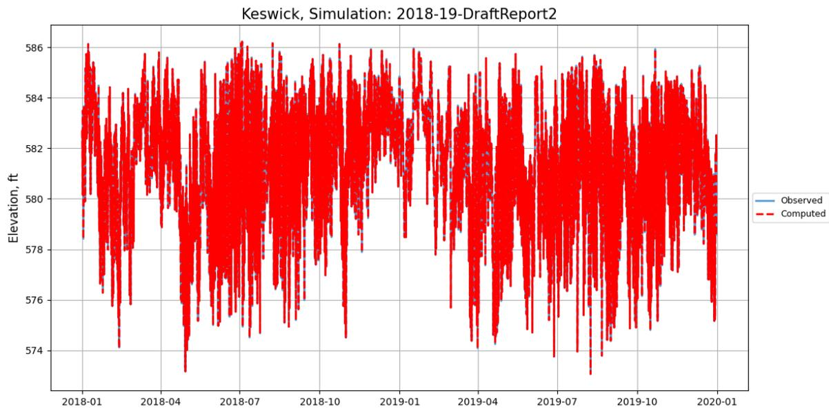
Figure 4-44. Keswick Reservoir simulated and observed water surface elevation, 2018-2019.
