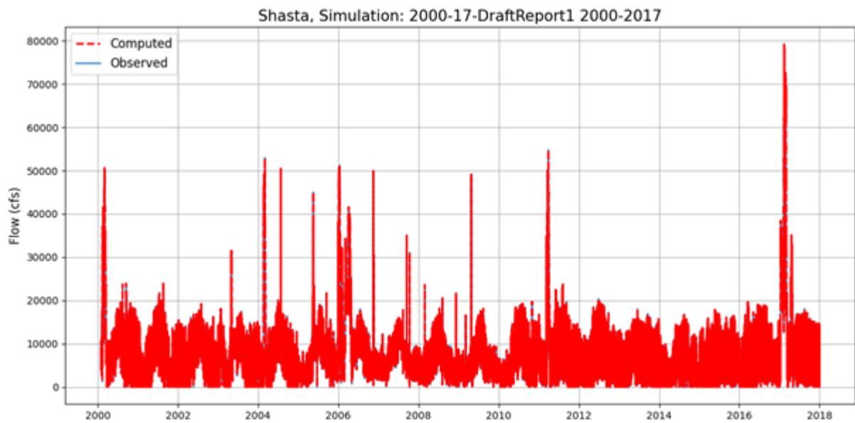
Figure 4-11. Shasta Lake simulated and observed out flow, 2000-2017.
