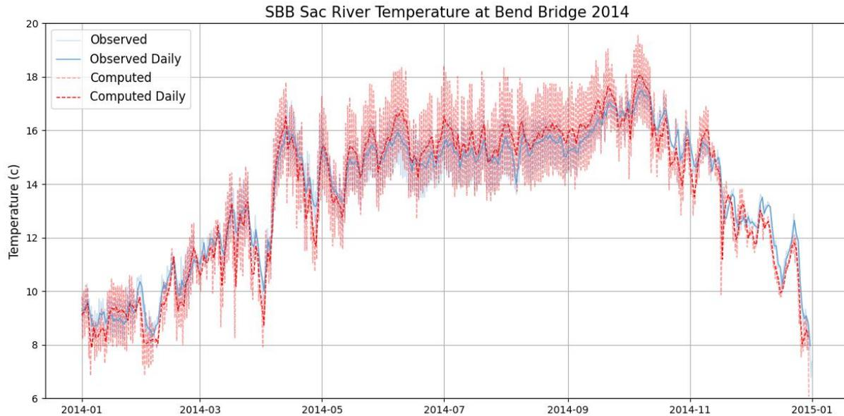
Figure 4-36. Simulated and observed temperatures at BND: 2014.
