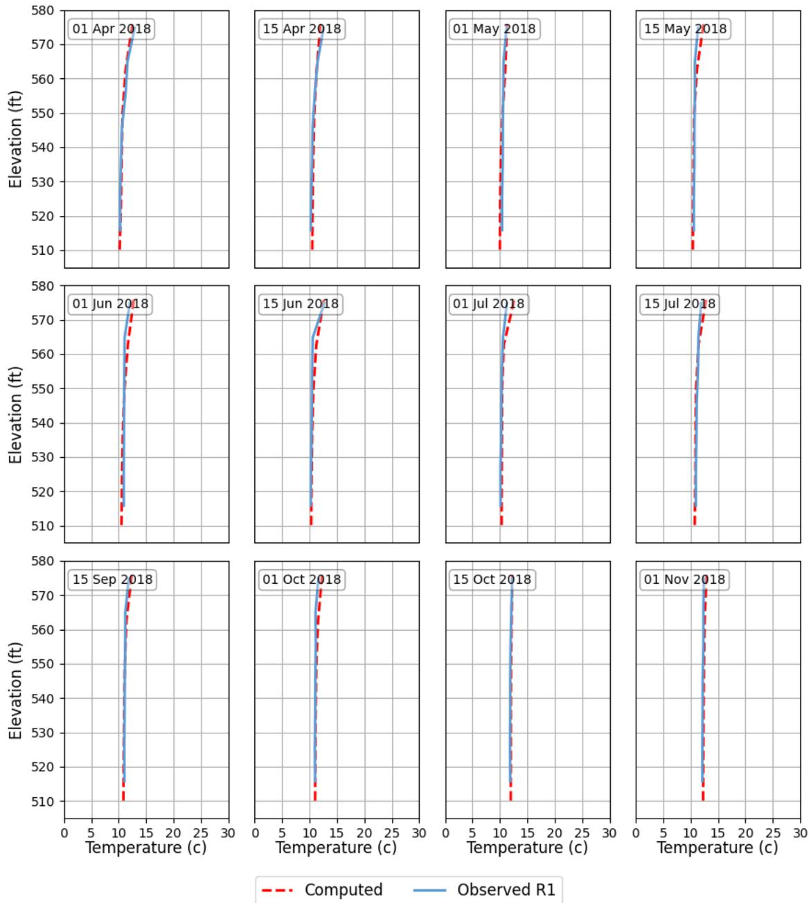
Figure 4-45. Keswick Reservoir simulated and observed temperature profile comparisons, 2018. Profiles data are collected approximately 0.1 miles upstream from dam (1/2).
