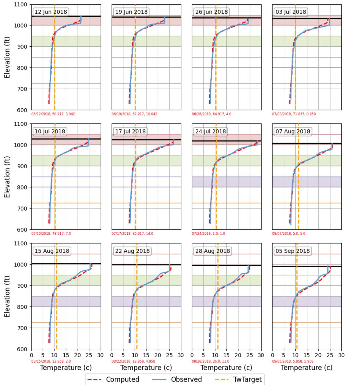
Figure 4-40. Simulated and observed temperature profiles and TCD gate positions during 2018 (2/3).
