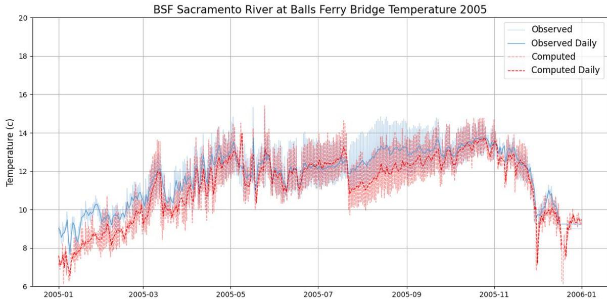
Figure 4-29. Simulated and observed temperatures at BSF: 2005.
