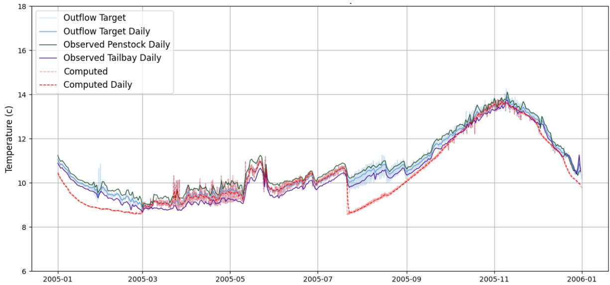
Figure 4-15. Shasta Lake daily simulated and observed temperatures at Shasta Dam, 2005.
