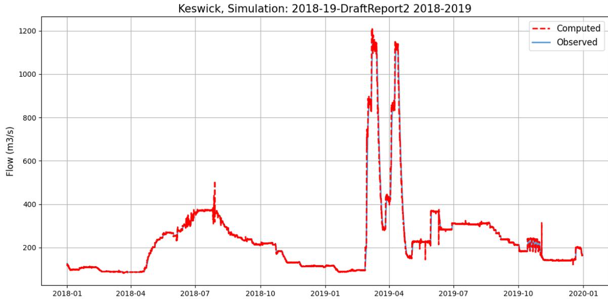
Figure 4-43. Keswick Reservoir simulated and observed flow through Keswick Dam, 2018-2019.
