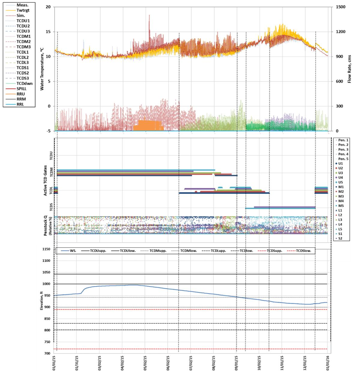
Figure 4-4. Shasta Lake simulated temperature vs. target temperature & measured temperature, and simulated outflows (top), Shasta Lake the TCD active gates and relative percentage of total outflow through penstocks (middle), Shasta Lake water surface elevation and the TCD gate elevations (bottom): 2015.
