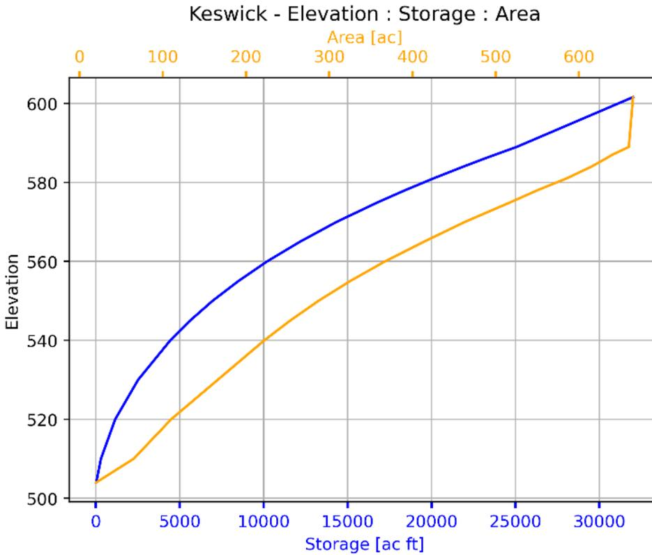
Figure 3-5. Keswick Reservoir elevation-storage and elevation-area curves.
