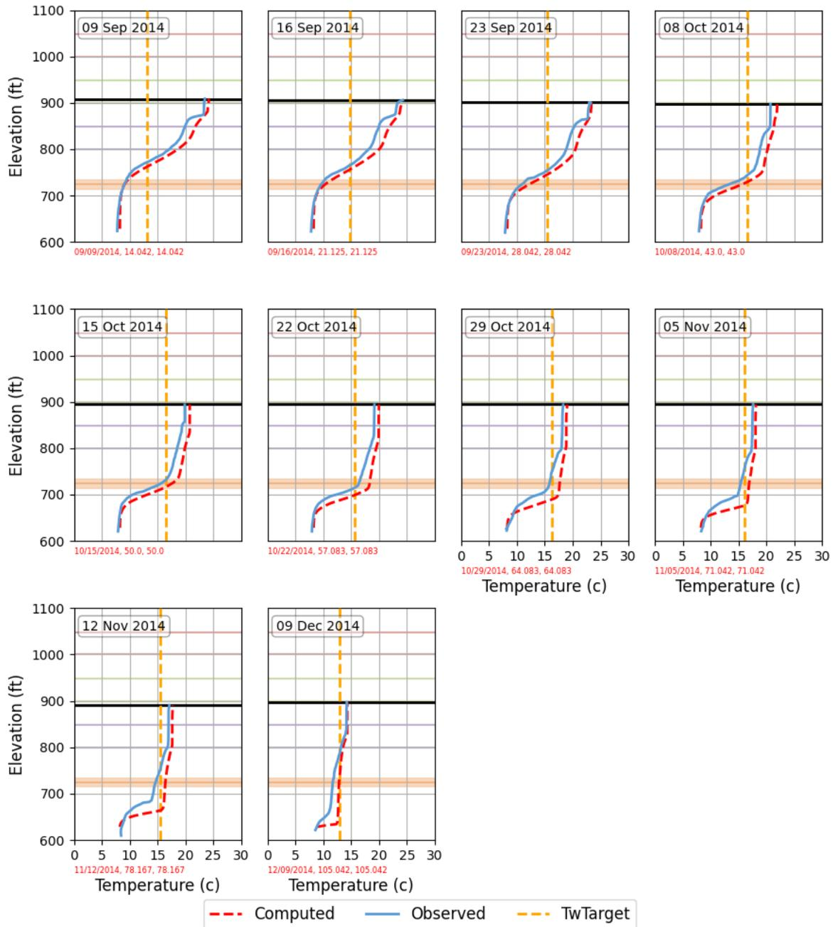
Figure 4-13. Simulated and observed temperature profiles and TCD gate positions during 2014 (2/2).
