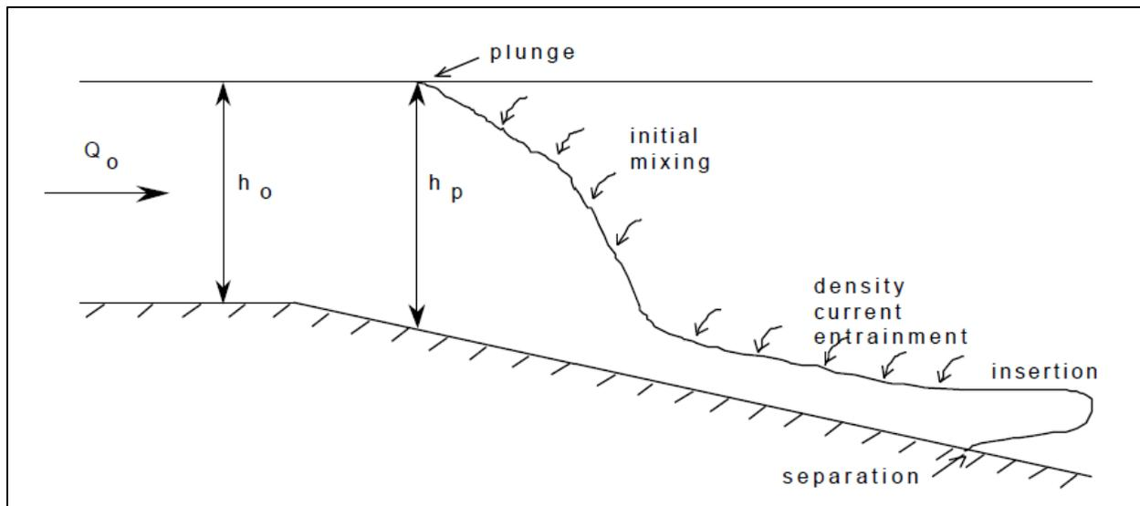
Figure 3-4 Schematic of entrainment for an interflow (from Fleenor (2001))
