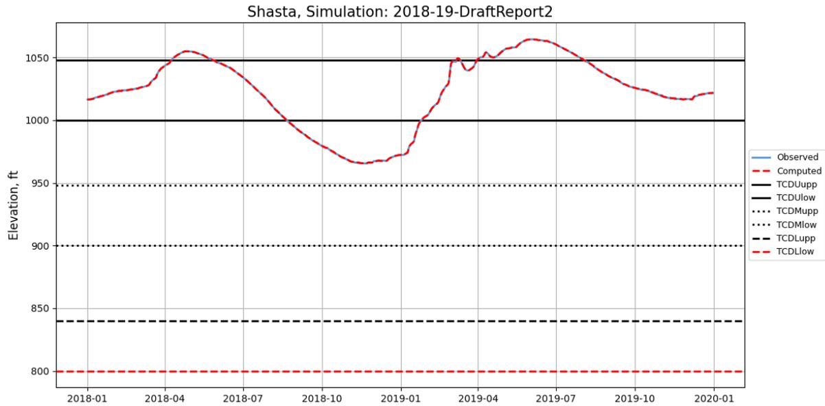
Figure 4-37. Shasta Lake simulated and observed water surface elevation, with TCD gate elevations, 2018-2019.
