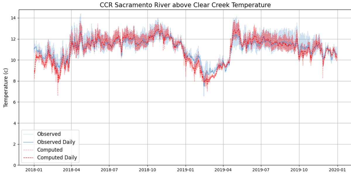
Figure 4-49. Simulated and observed temperatures at CCR: 2018-2019
