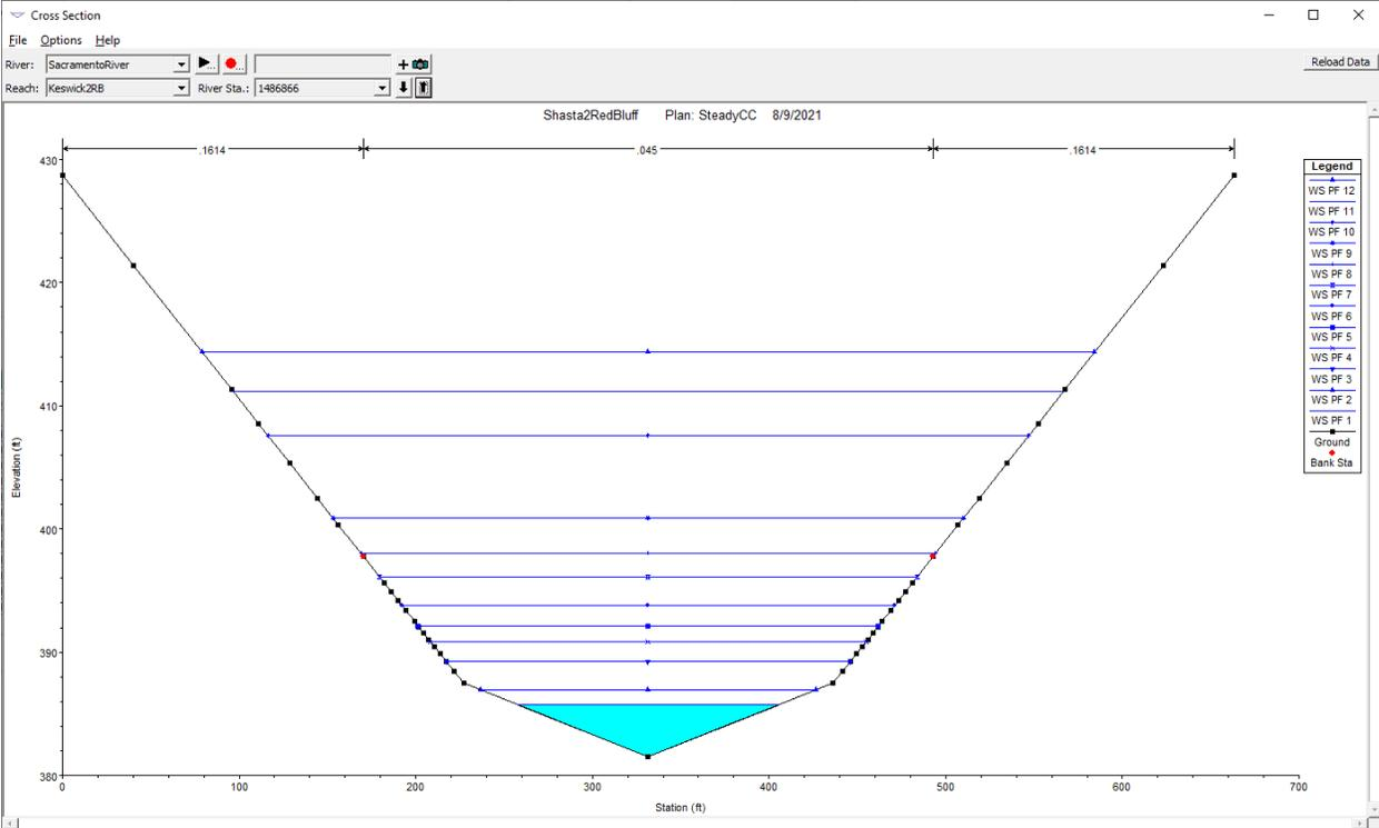
Figure 3-7. HEC-RAS display of an exported HEC-5Q cross section, representing a section of the Sacramento River below Clear Creek.
