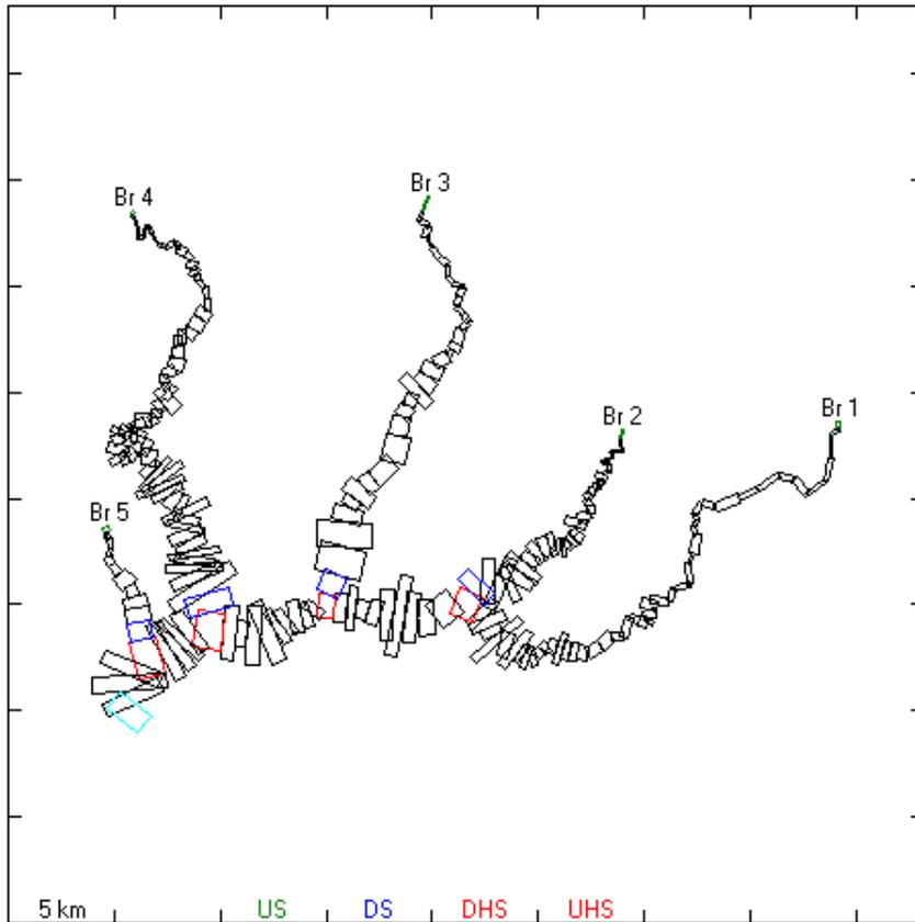
Figure 3-1. Shasta Lake model grid (plan view). The furthest upstream segments of each branch are shown in green (nearest the branch label); terminal downstream segments of Branches 2 through 5 are blue; “connection” segments for the tributaries to the main branch are red; and furthest downstream segment of the entire model grid, just above Shasta Dam, is cyan (bottom left).
