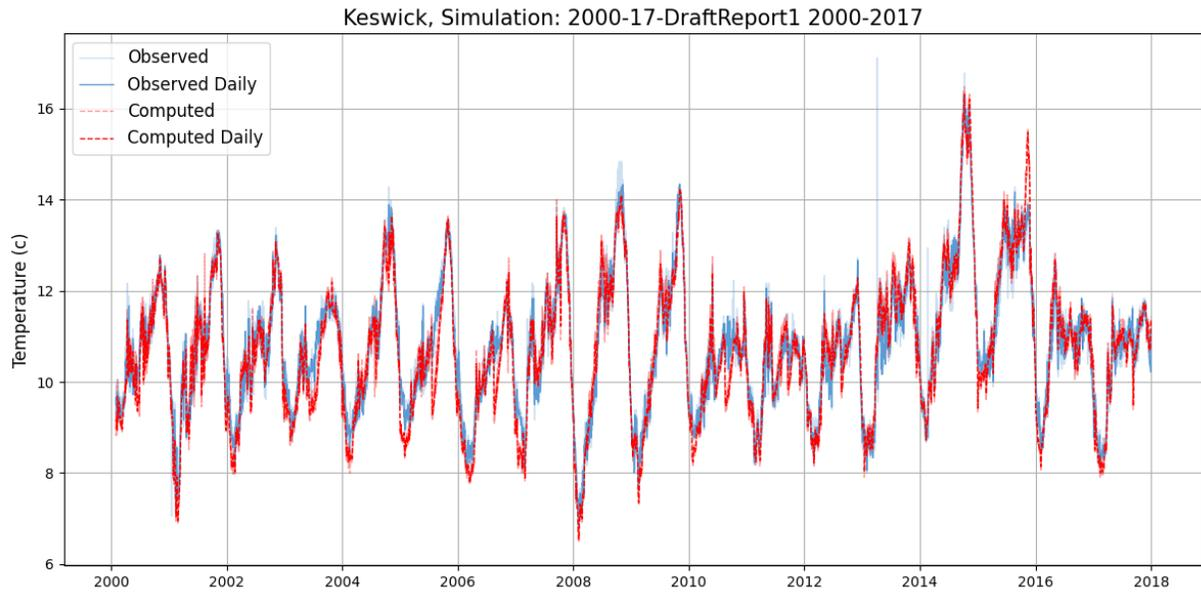
Figure 4-21. Simulated and observed outflow temperatures from Keswick Dam: 2000-2017.
