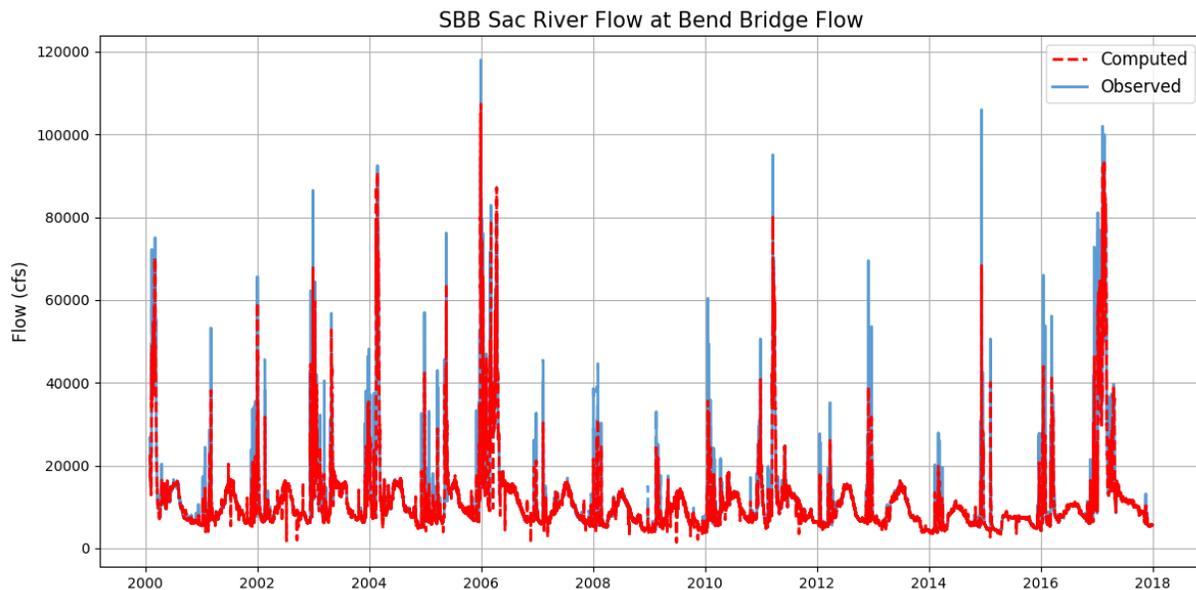
Figure 4-23. Simulated and observed hourly flows at Bend Bridge: 2000-2017.
