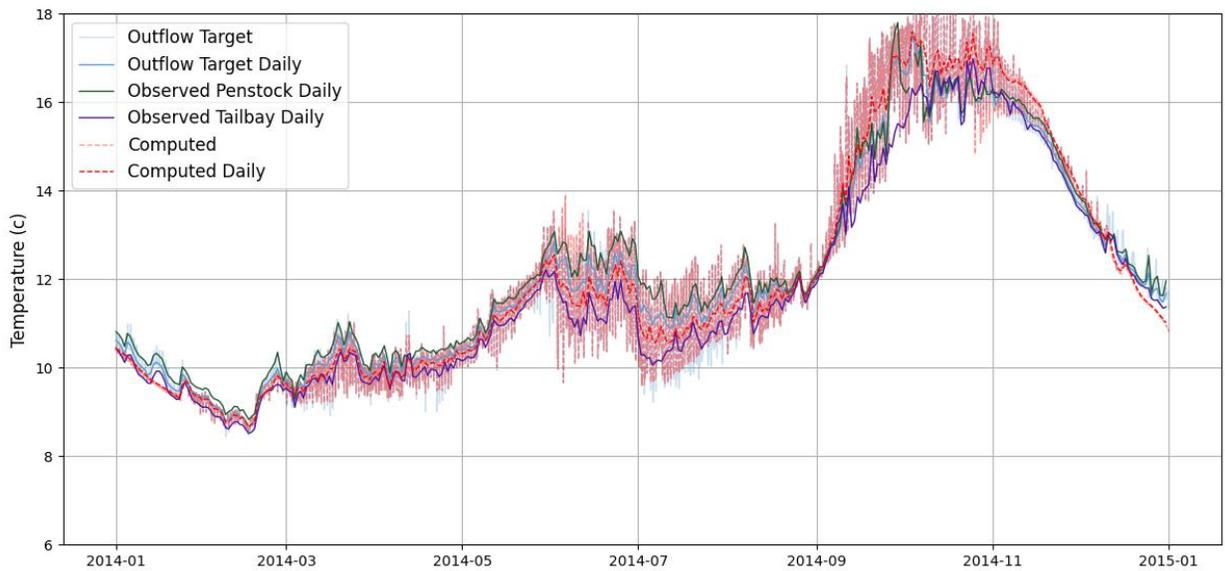
Figure 4-16. Shasta Reservoir hourly simulated and observed temperatures at Shasta Dam, 2014.
