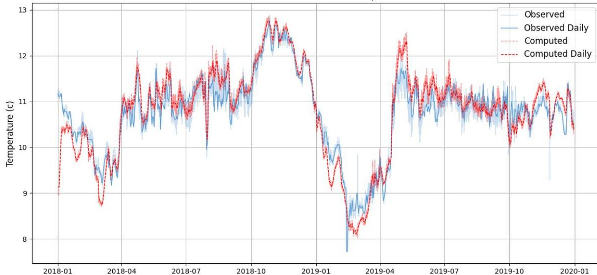
Figure 4-47. Simulated and observed outflow temperatures from Keswick Dam: 2018-2019.
