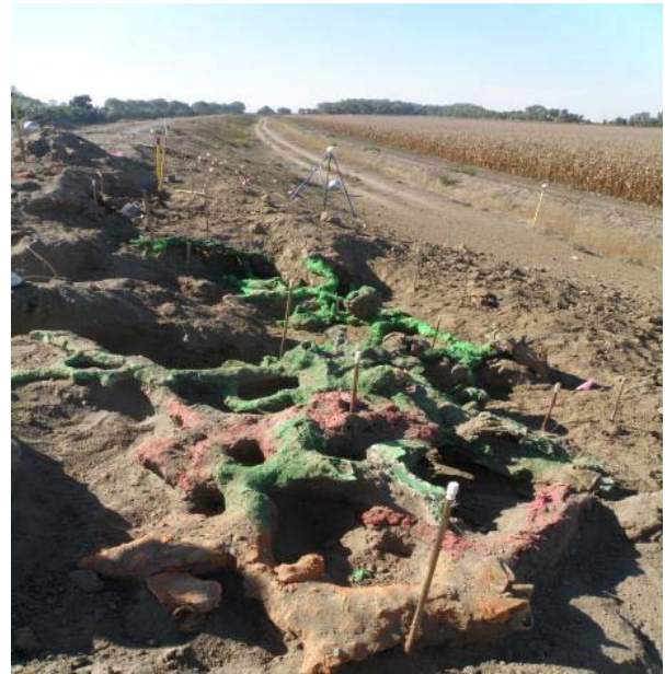
Post excavation - site with grouted excavated burrows
