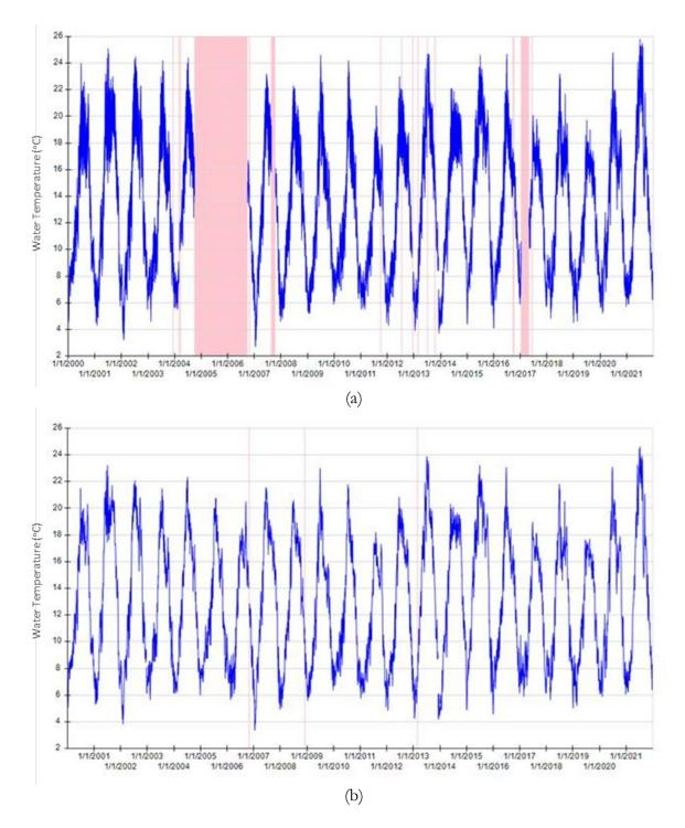
Figure 3-2. DMS example of data gap graphical reporting tool (a) to identify data gaps in a record and (b) for final data set review.
