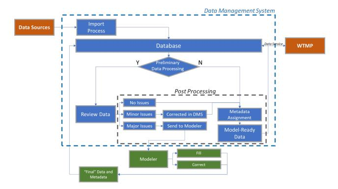
Figure 3-3. Flow chart of DMS showing Post-Processing step and the role of modeler filling/correcting data to address gaps or erroneous data and meta-data assignments.
