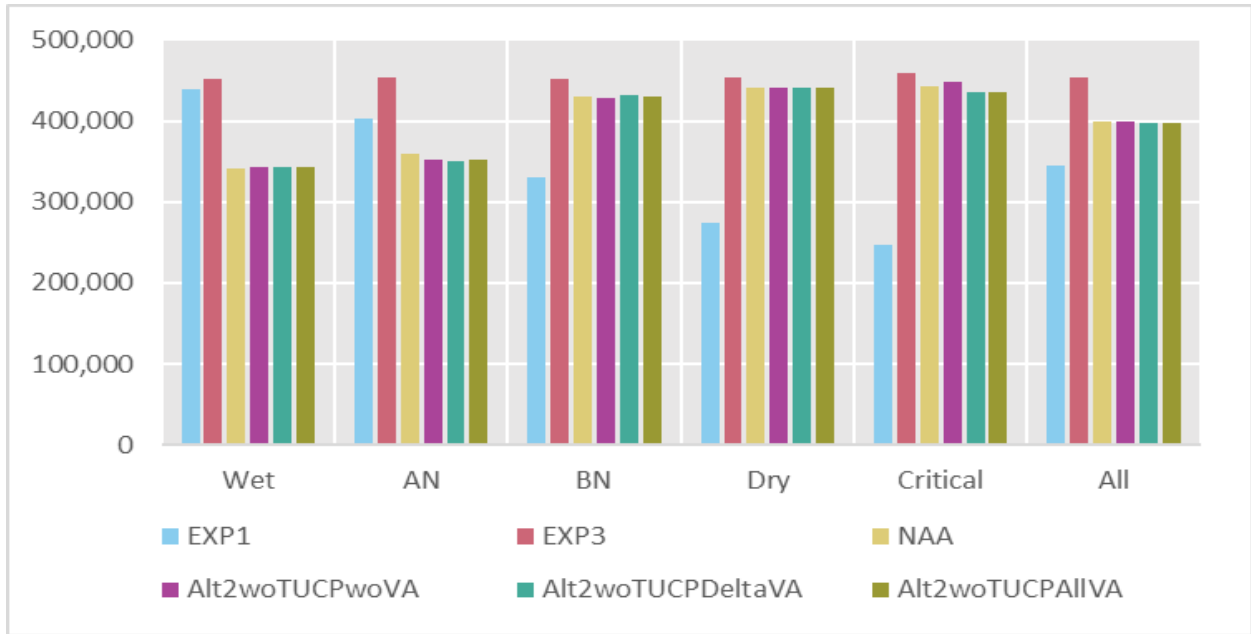
Figure 6-4. Mean Weighted Usable Area for Segments 5+6 by Water Year Type, Spring-run Spawning in the Sacramento River
